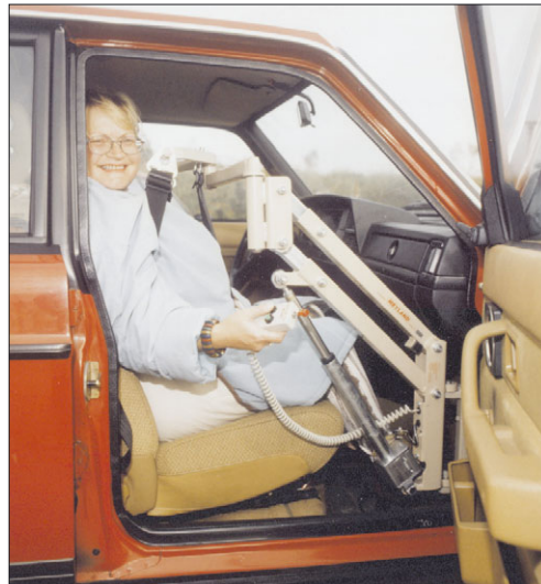
The permanent lift console is the only visible part in the car when the lift is not in place.
